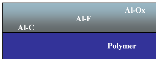
Figure 3.7. Composition diagram of aluminum adlayer on aParylene AF-4 film.
