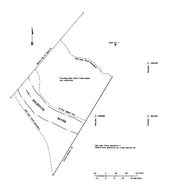
FIGURE 4.--Overlay to National Park Service drawing No. 149/80018 showing flood boundaries for the Soleduck River.
