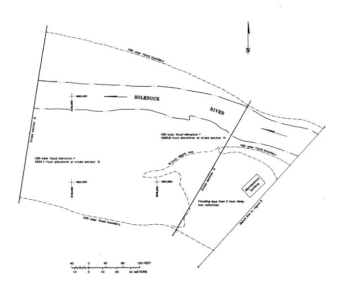
FIGURE 7.--Overlay to National Park Service drawing No. 149/80018 showing flood boundaries for the Soleduck River.
