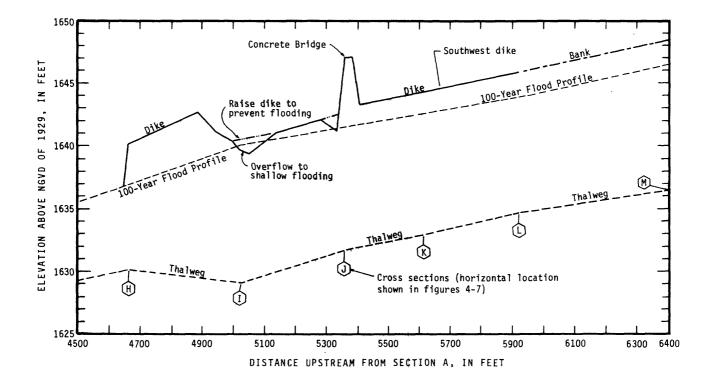
FIGURE 8.--The 100-year flood profile of the Soleduck River along the dike protecting the Sol Duc Hot Springs.
