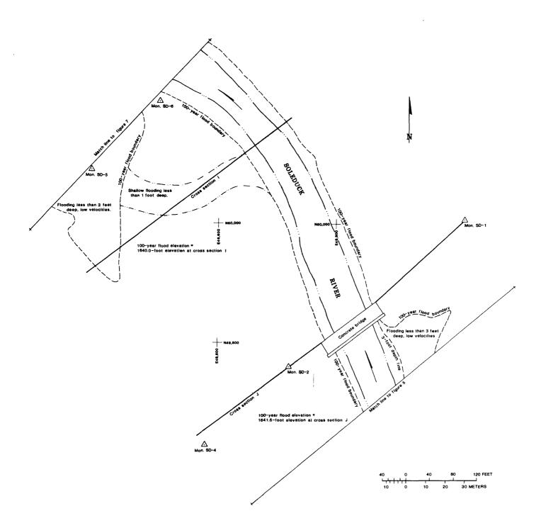
FIGURE 6.--Overlay to National Park Service drawing No. 149/80018 showing flood boundaries for the Soleduck River.
