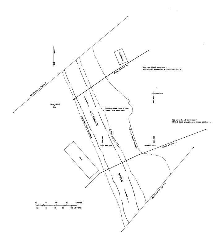
FIGURE 5.--Overlay to National Park Service drawing No. 149/80018 showing flood boundaries for the Soleduck River.
