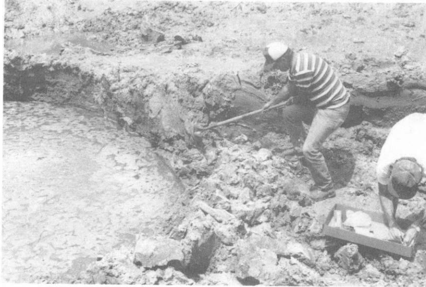
Figure A5. Obtaining samples from organic layer at about 12 feet. Organic layer right at water line.
