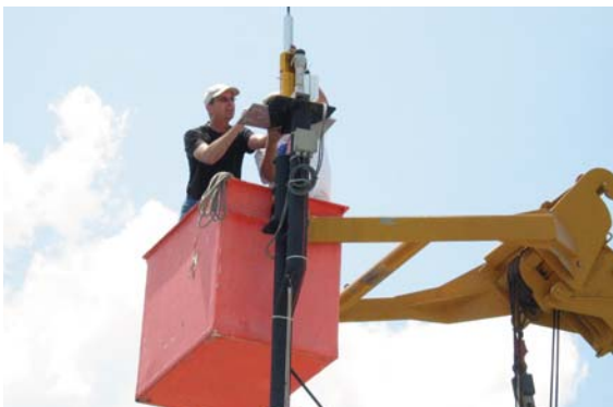
Project co-investigator Byron Blomquist mounts inlets and a sonic anemometer on the jackstaff of the National Oceanic and Atmospheric Administration Research Vessel Seward Johnson . The atmospheric pressure ionization mass spectrometer laboratory container is in the foreground. Credit: Barry Huebert, University of Hawaii
