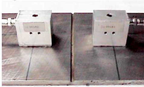
(a) Through transmission mode; EMATs are 3 in. away from each other and 1.5 in. from center groove.
