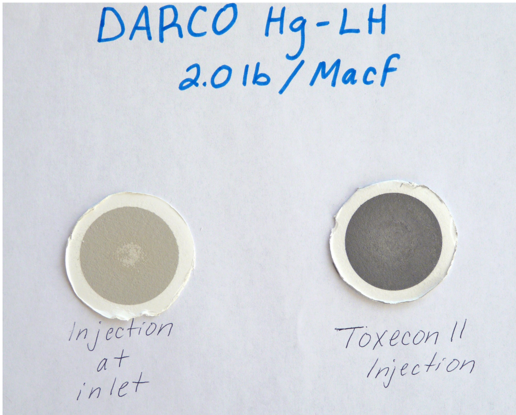
Figure 3-23. Photograph Comparing Method 17 Filters Collected during Toxecon™ II and Injection Upstream of the ESP
