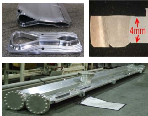
Figure 3: Machined extrusion end and the mating adapter plate (top left). Micrograph of the welds (top right), and the completed multipole chamber.
