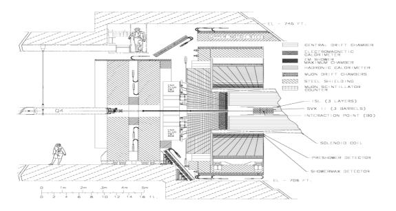
Figure 7: The CDF Run II Detector
