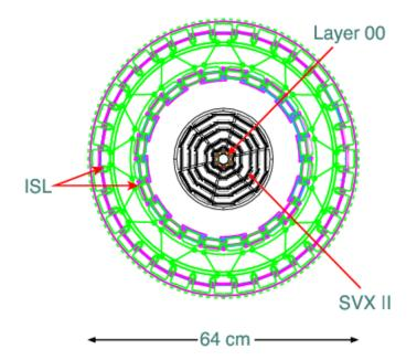
Figure 8: An end view of the CDF Run II silicon detectors.
