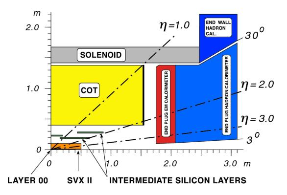
Figure 9: An r-z view of the CDF Run II tracking detectors.
