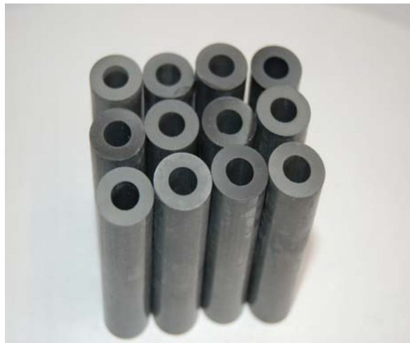
Fig. 3: SiC tubular supports sintered at 1700°C for 3 h.
