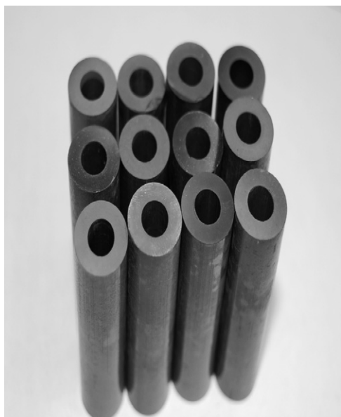
Fig. 1. SiC tubular supports sintered at 1700 °C for 3 h.
