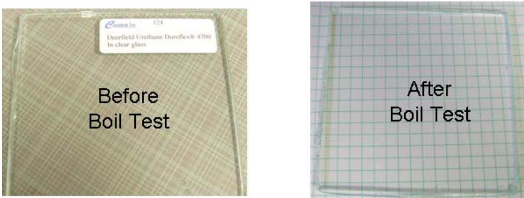
Figure 3. Before and after photographs of 1.5 year room-temperature aged thermoplastic polyurethane (TPU) RF-laminated sample, subjected to boil test – 2 hours in boiling water. The sample passed the test, retaining defect free clarity after boiling, with no development of bubbles, delamination, or haze.
