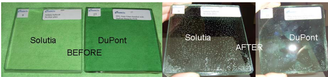
Figure 4. Before and after photographs of 2 year room-temperature aged PVB test samples, subjected to bake test at ~110 °C for 1 hour. The laminates appeared clear and defect free before the bake test and exhibited no delamination in the 2 years since lamination. After a 1 hour bake test, the samples developed numerous bubbles indicative of dissolved air. No hazing or delamination was observed, indicating otherwise strong adhesion to the glass.
