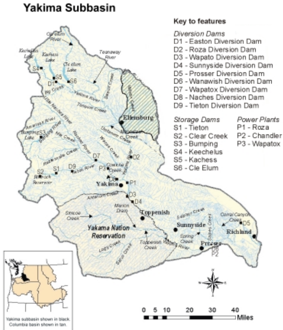
Figure 2.1. Map of the Yakima Subbasin showing major storage, diversion, and hydroelectric dams (Source: Draft Yakima Subbasin Summary, 2001).
