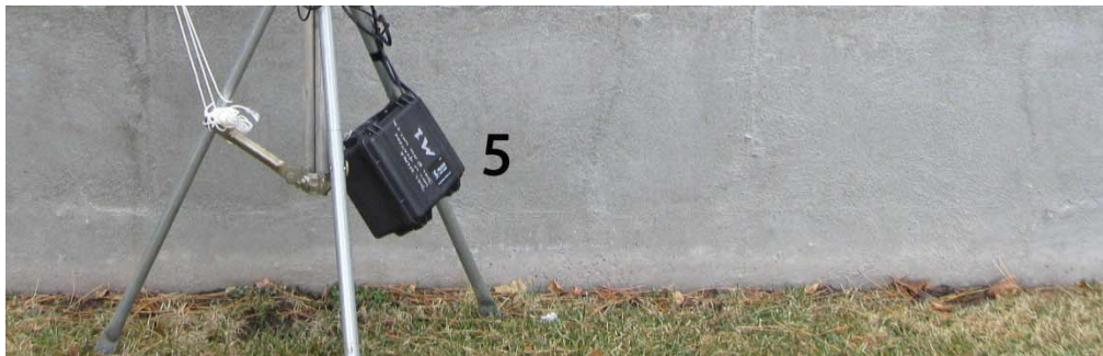
Figure 4: An example of one of the met stations. 1) Sonic Depth Sensor. 2) 5W Solar Panel. 3) Temperature Probe housed inside a radiation shield. 4) Radiation Sensor. 5) Data-Logger housed inside a waterproof Pelican Case.
