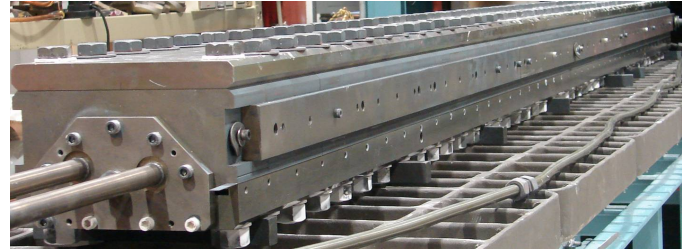
Fig. 5. LQ reaction fixture with top plate after heat treatment.
