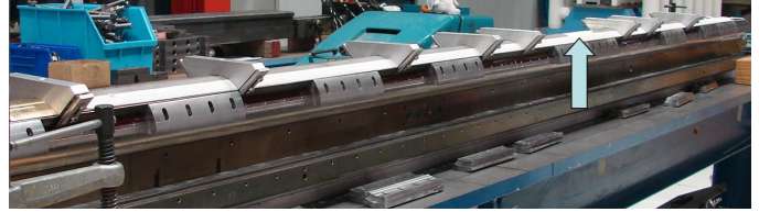
Fig. 4. LQ coil on winding mandrel with central pole parts removed after curing (the arrow points to the missing pole parts).
