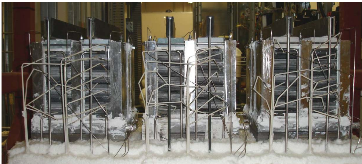
Figure 25. HTE ILS hot zone with three modules installed.
