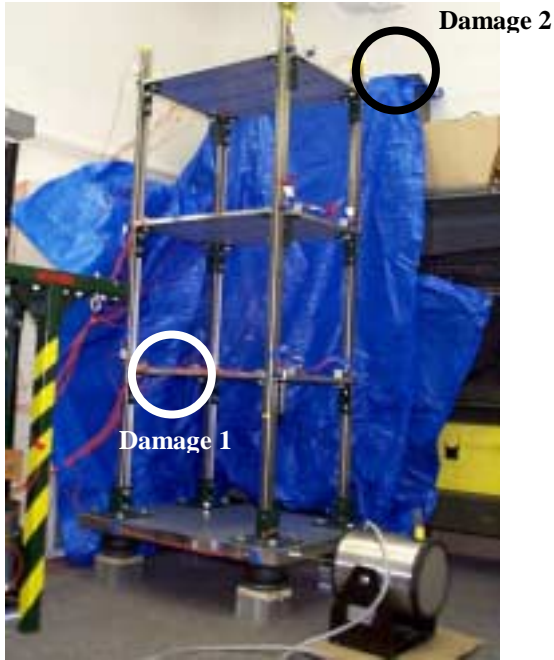
Figure 1. Photo of the full test structure.
