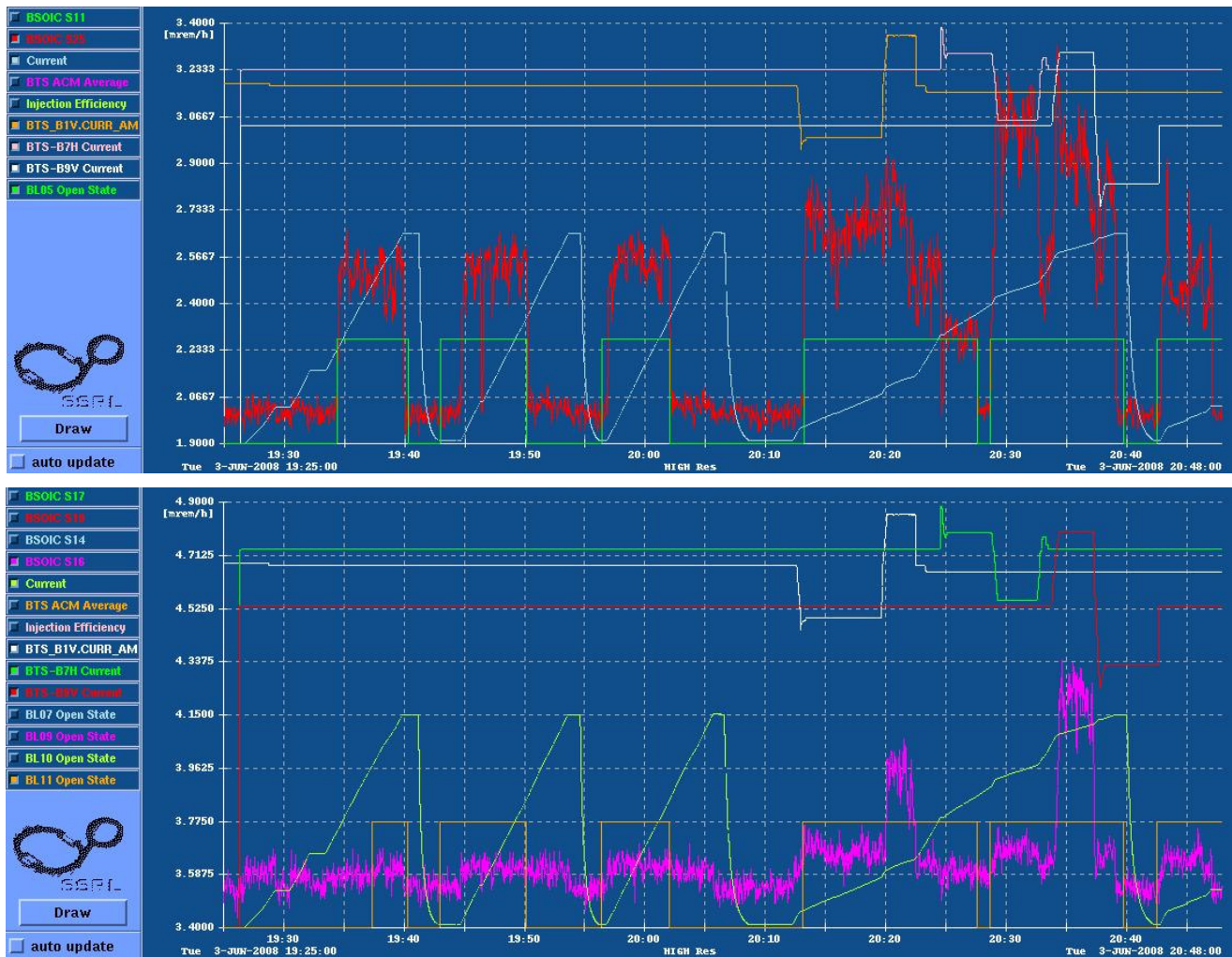
Fig.2 – Typical results from first Top-Off tests for BL 5 (top) and BL 11 (bottom). Three high-efficiency injections (left) were followed by one low-efficiency injection. The units on the vertical axis correspond to the radiation measurements of the BSOIC (red on top, pink on bottom).
