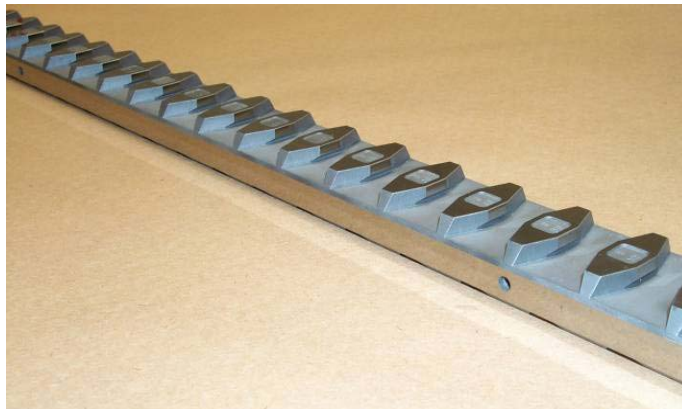
Figure 3: Photograph of a macroscopic step bar; the pitch between flats is 30mm.
