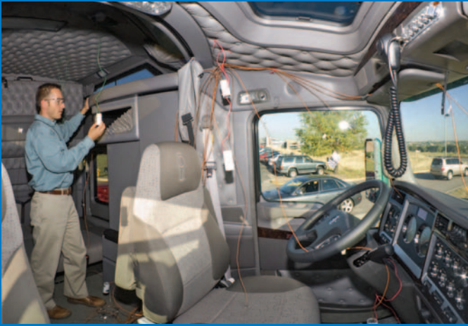
NREL Senior Project Leader Ken Proc examines sensors that measure the outside ambient temperature and compare it to the temperature in truck cabs. Credit: Pat Corkery PIX 16811
