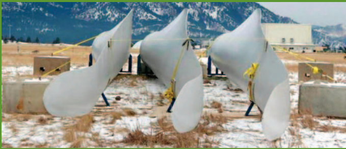
Blades of the General Electric 1.5 MW turbine are being stored outside on cradles this winter at the National Wind Technology Center. They are secured with large concrete blocks to prevent them from being damaged during high winds and storms. Credit: Jim Green/PIX 16179
