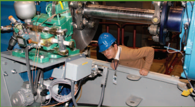
NREL senior engineer Shuangwen Sheng inspects the monitoring system for the long-term gearbox reliability study at the National Wind Technology Center. Credit: Joseph B. Verrengia/PIX 16867
