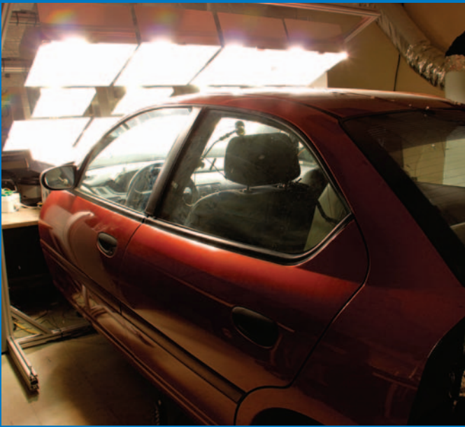
Solar lights in NREL's Vehicle Climate Control Laboratory help simulate heating of cars and assist researchers in finding more efficient ways to cool cars. Credit: Heather Lammers/PIX 16869
