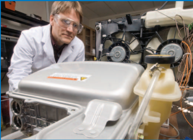
NREL senior engineer Ken Kelly monitors testing of a Toyota hybrid system drive. Kelly's group is developing ways to transfer heat from the system's electronics in order to improve efficiency and extend the component's life. Credit: Pat Corkery/PIX 16586
