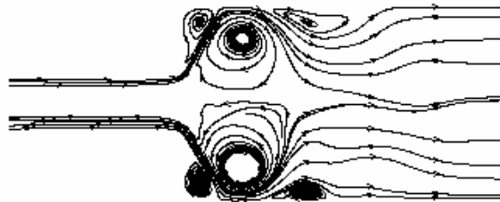
Figure 15. Two-dimensional view of mean streamline profiles of the flow around the popper valve in sudden-expansion configuration.
