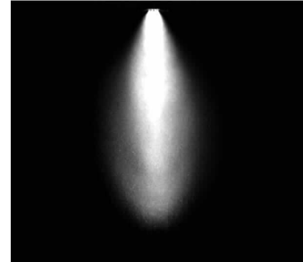
Figure 1. Spray with 40^\circ spray angle / 0^\circ offset angle
