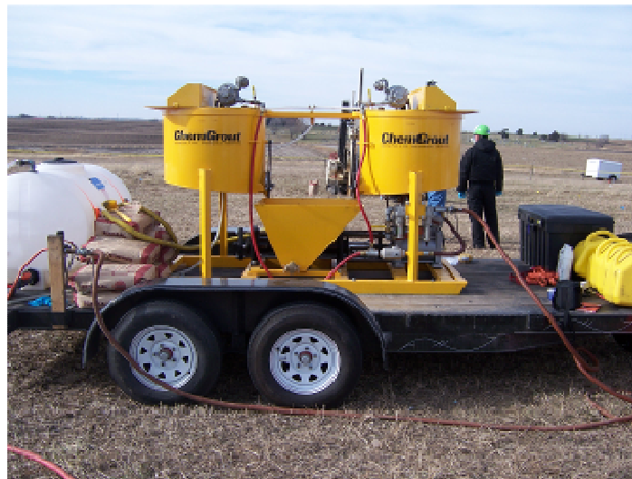
Figure 6. Chem Grout Pump
