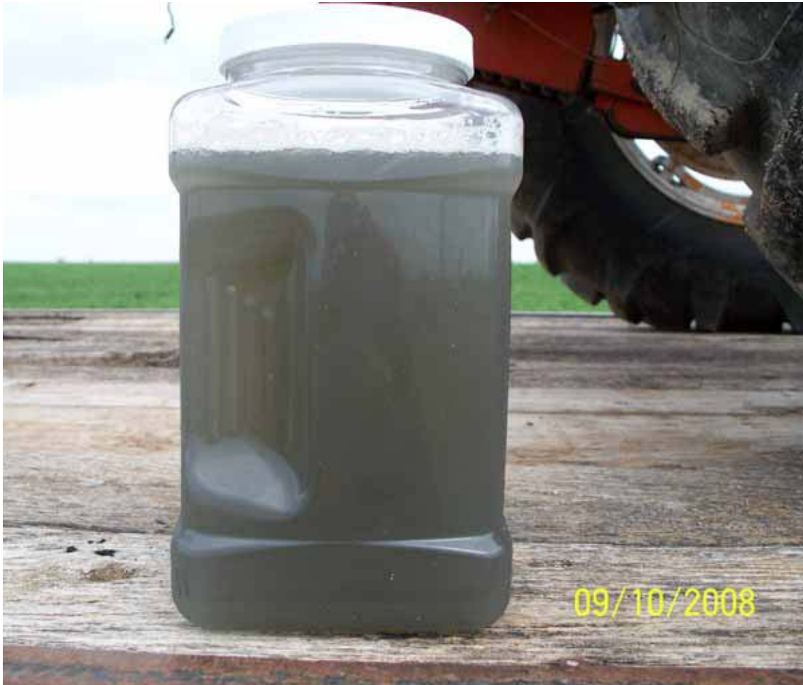
FIGURE 4.8 Appearance of groundwater collected from monitoring well MW02 during the September 2008 post-injection sampling event.
