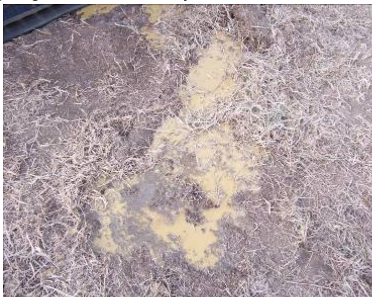
Figure 12. Daylighting of Thin EHC-A Slurry at PT-1
