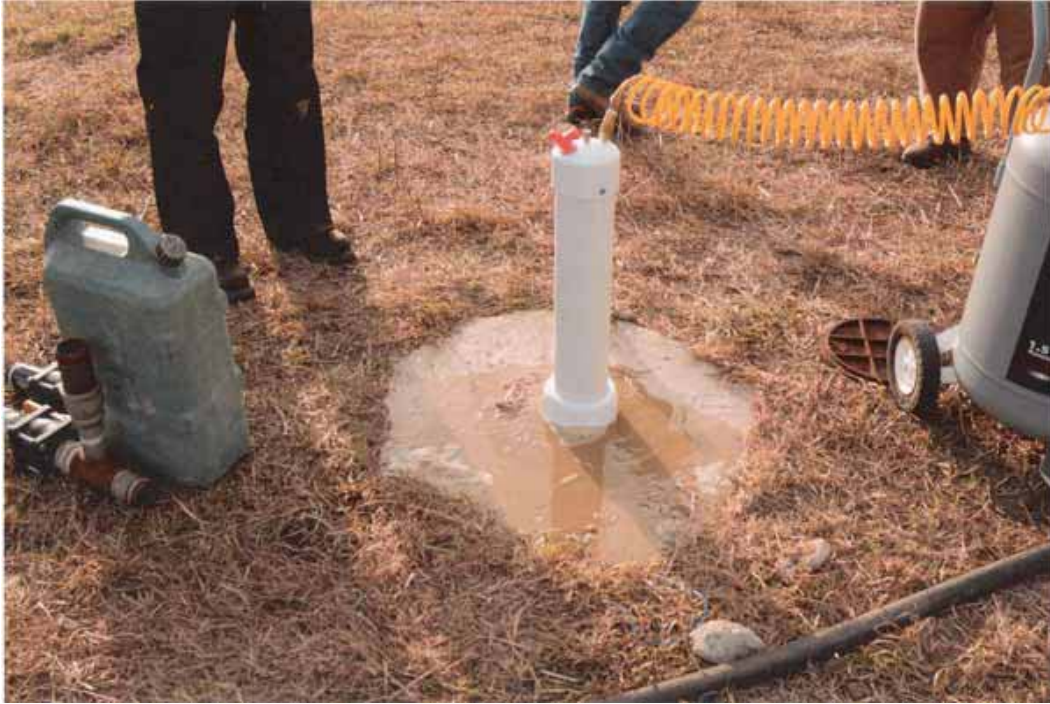
Daylighting of EHC-A solution observed at monitoring well MW02.
