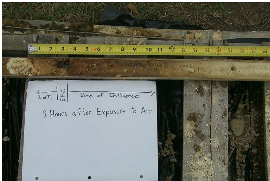
Figure 4. Photograph of a soil core, from 30 ft to 33 ft bgs, showing a 1-inch fracture
