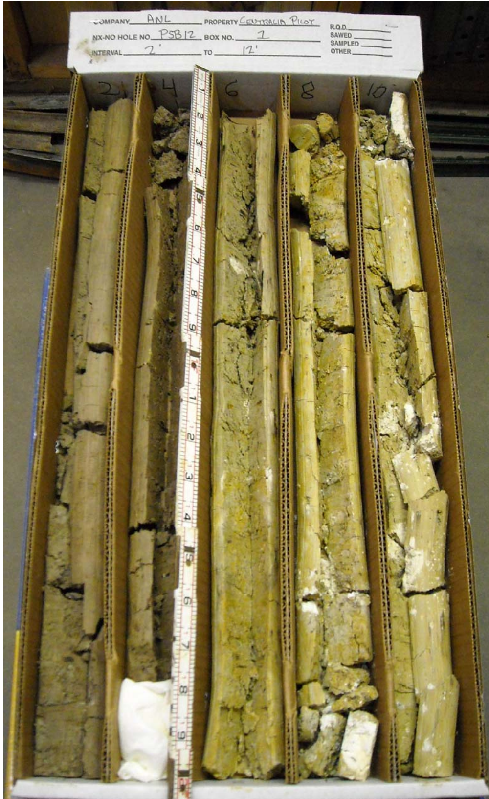
FIGURE B.3 Photographs of the soil core collected from boring PSB12 approximately two weeks after injection, in December 2007.
