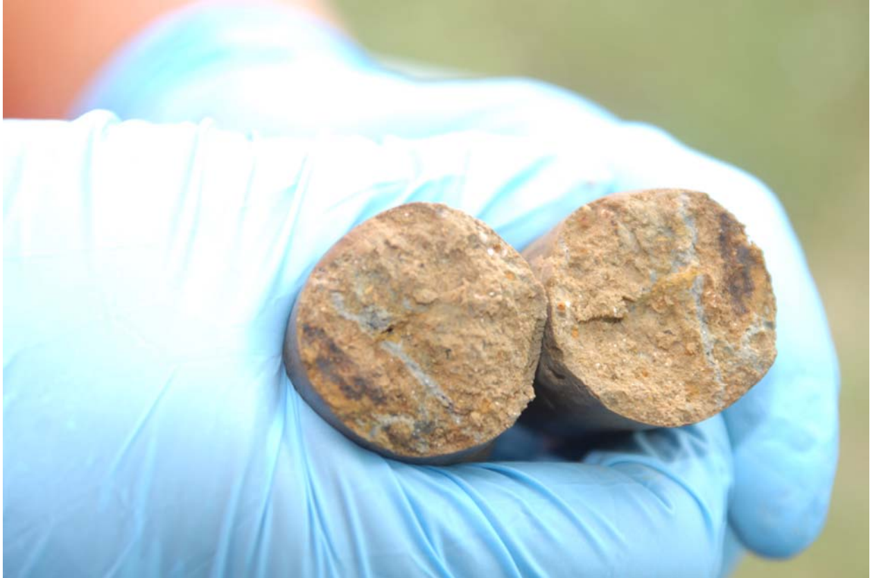
FIGURE 3.5 Appearance of EHC material along small, isolated fractures in the soil core recovered at 21 ft BGL at post-injection soil coring and sampling location PSB13.
