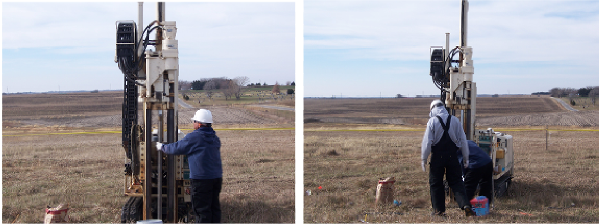
Figure 5. Direct Push Rig Used for EHC Injections
