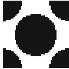
Fig. 4 A representative elemental volume for the periodic array of small circles.
