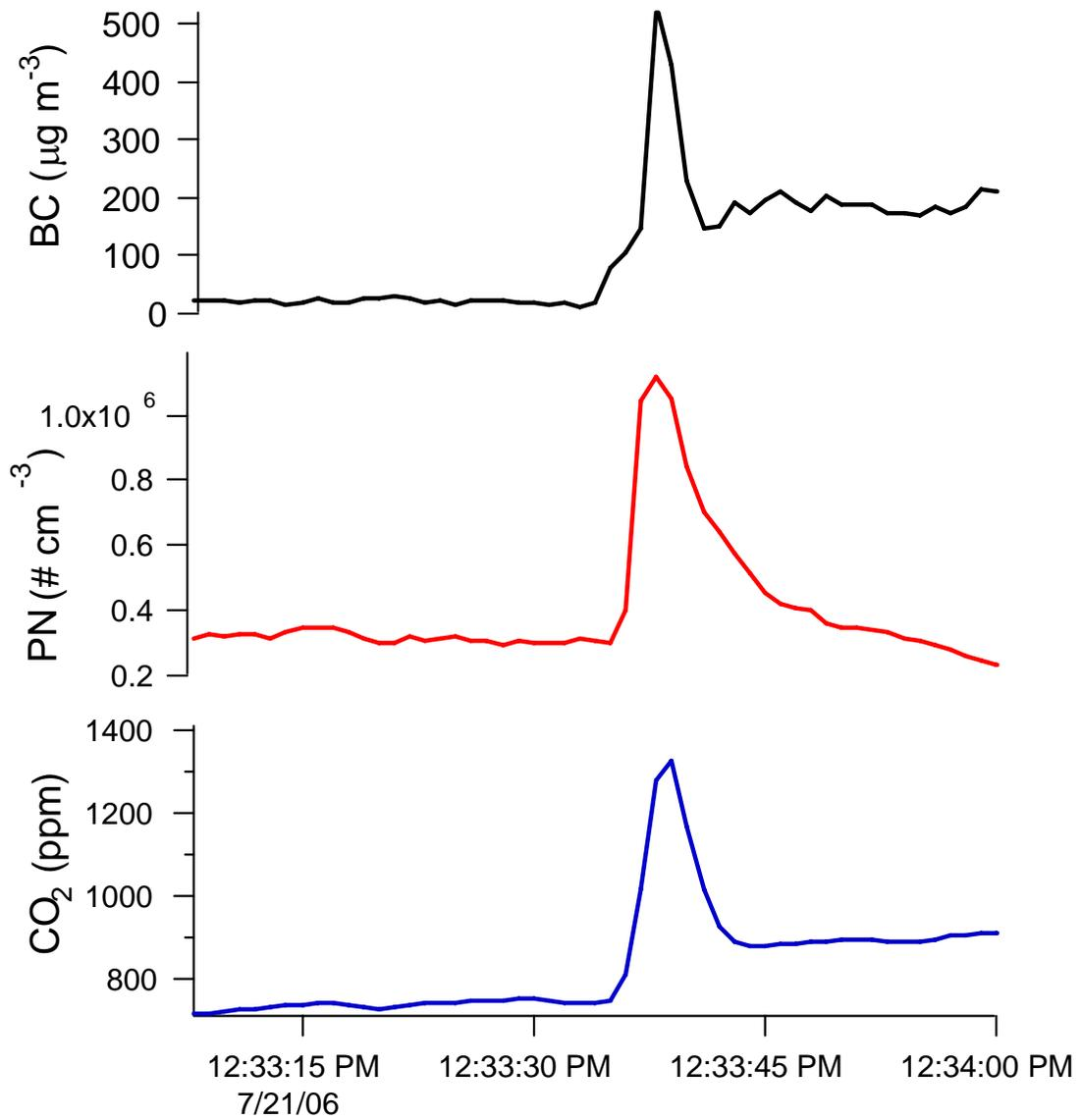
Figure 1. Measured black carbon (BC), particle number (PN), and CO<sub>2</sub> concentrations in the exhaust plume of a passing HD truck.
