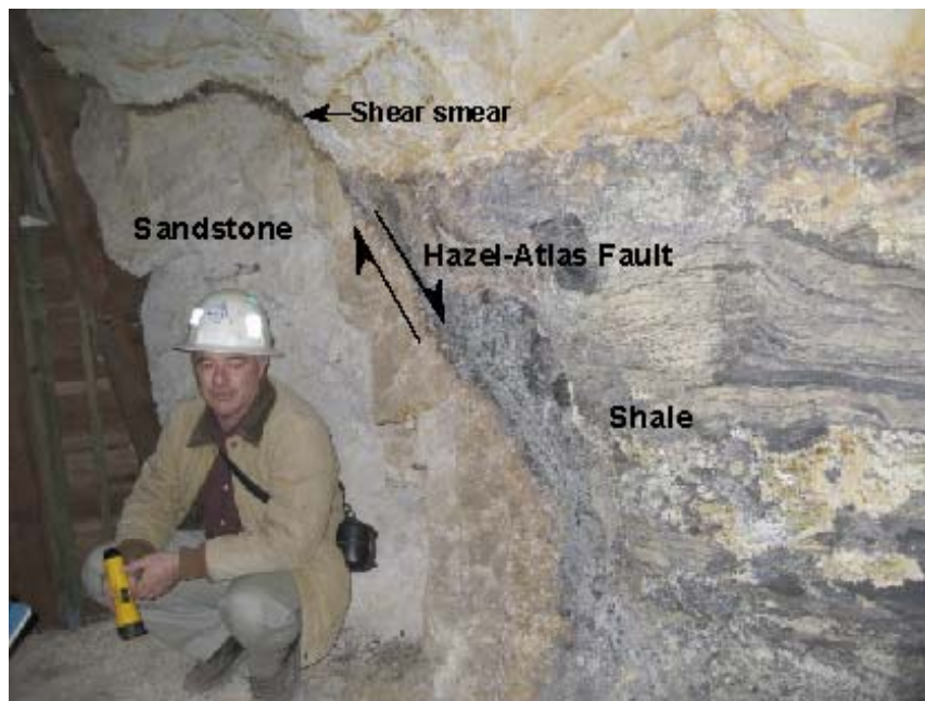
Figure 2-15 Picture showing the Hazel-Atlas fault in the Black Diamond Mine, Antioch, CA
