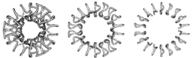
FIG. 8: Top view of modular coils constructed for configurations (b) with A = 4 , (d) with A = 6 , and (e) with A = 8 of Figure (6). Coil winding surfaces have been constructed such that the inboard midplane is displaced by 0.6a whereas the outboard miplane is displaced by 1.2a , where a is the plasma minor radius, with interpolation made for locations in between. In all cases, there are three types of coils for each half-period for a total of 18 coils.
