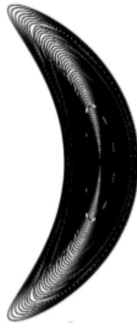
FIG. 4: Contours of flux surfaces for the configuration shown in Figure (1)(d) at \beta = 4\% from a PIES calculation showing the configuration has good surface quality despite the existence of rational values in the iota profile.
