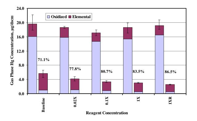
Figure 2-1 – Mercury Removal and Speciation with Alternate Reagent
