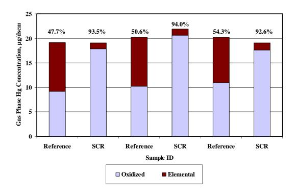
Figure 2-3 – Effect of SCR Catalyst on Mercury Speciation
