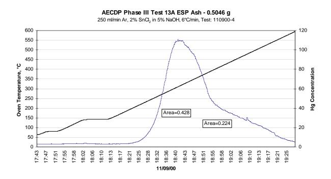
Figure 3-16 – TSC for ESP Ash (Sorbent Injection)
