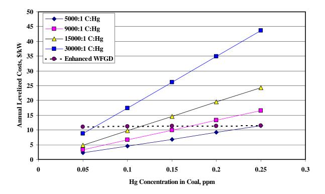
Figure 2-8 – Annual Cost Comparison for Wet FGD and Activated Carbon
