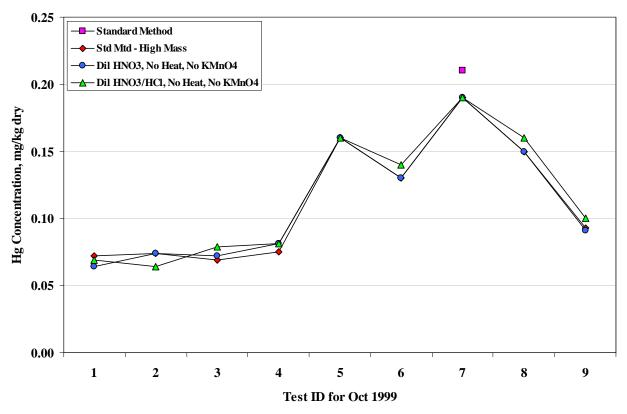
Figure 3-1 – Hg Concentrations in Wet Scrubber Hydroclone Underflow Slurry
