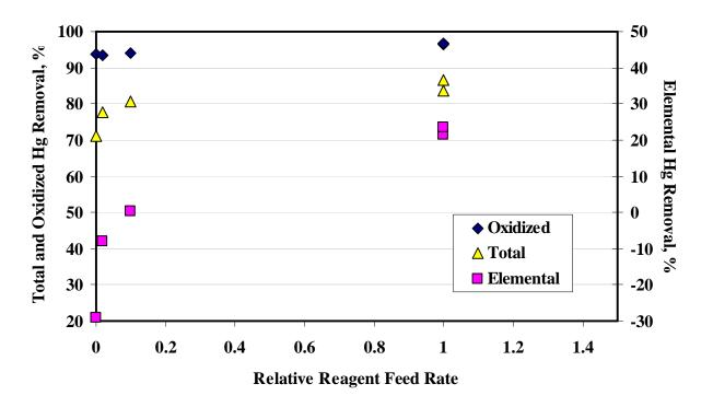
Figure 2-2 – Oxidized, Elemental and Total Mercury Removal Results
