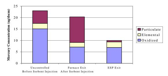
Figure 2-5 – Limestone Injection Mercury Capture at Ca/S = 0.35 mol/mol
