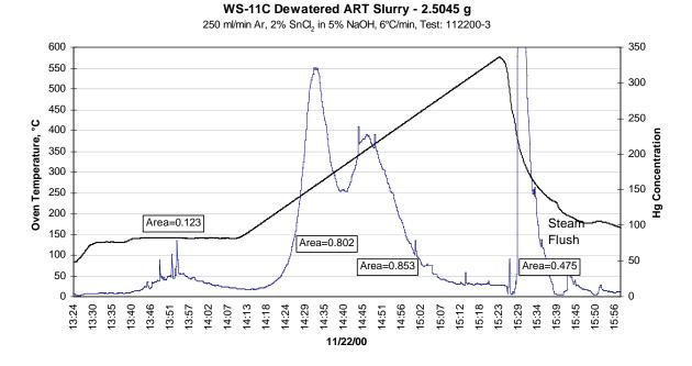
Figure 3-21 – TSC for AECDP Phase III Test 11C Wet FGD Sludge (App2)
