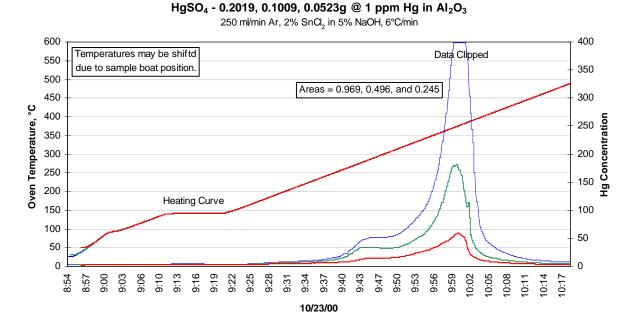
Figure 3-7 – Multiple TSCs for the HgSO4 Standard at Various Sample Weights
