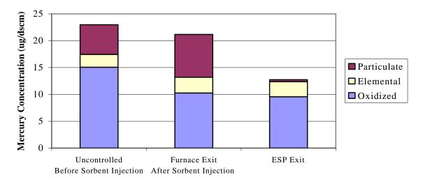
Figure 2-4 – Limestone Injection Mercury Capture at Ca/S = 0.04 mol/mol
