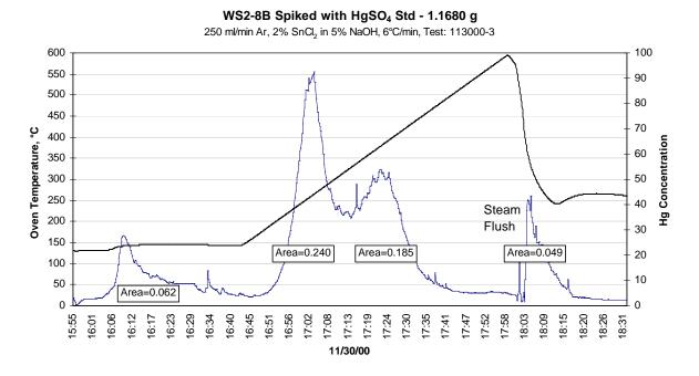
Figure 3-33 – TSC for MTI Wet FGD Slurry Spiked with HgSO₄ Standard
