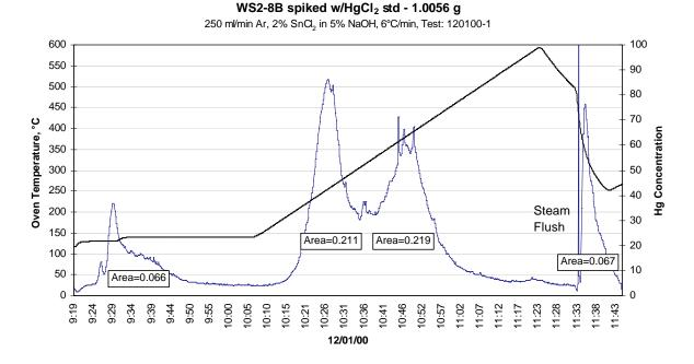
Figure 3-34 – TSC for MTI Wet FGD Slurry Spiked with HgCl<sub>2</sub> Standard
