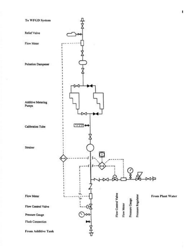
Figure 2-7 – Enhanced Wet FGD Equipment Schematic
