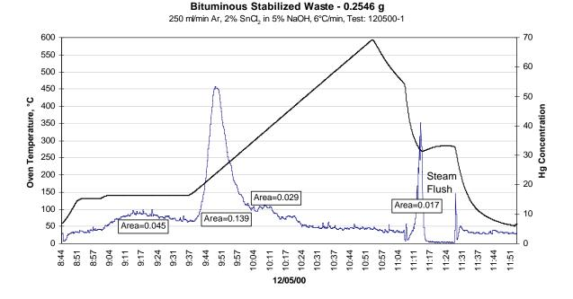
Figure 3-30 – TSC for an Eastern Bituminous Coal Landfill Waste
