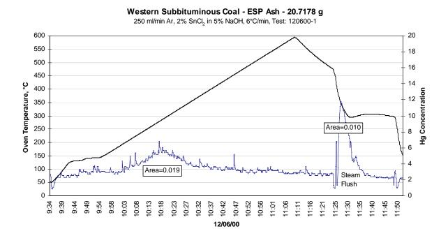
Figure 3-28 – TSC for a Western Subbituminous Coal Blend ESP Ash
