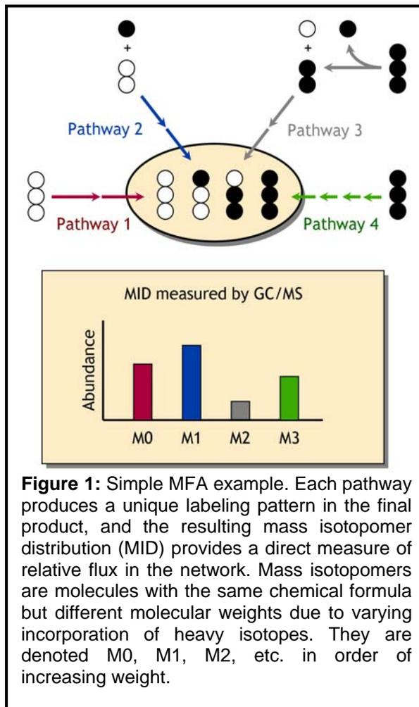
**Figure 1:** Simple MFA example. Each pathway produces a unique labeling pattern in the final product, and the resulting mass isotopomer distribution (MID) provides a direct measure of relative flux in the network. Mass isotopomers are molecules with the same chemical formula but different molecular weights due to varying incorporation of heavy isotopes. They are denoted M0, M1, M2, etc. in order of increasing weight.
