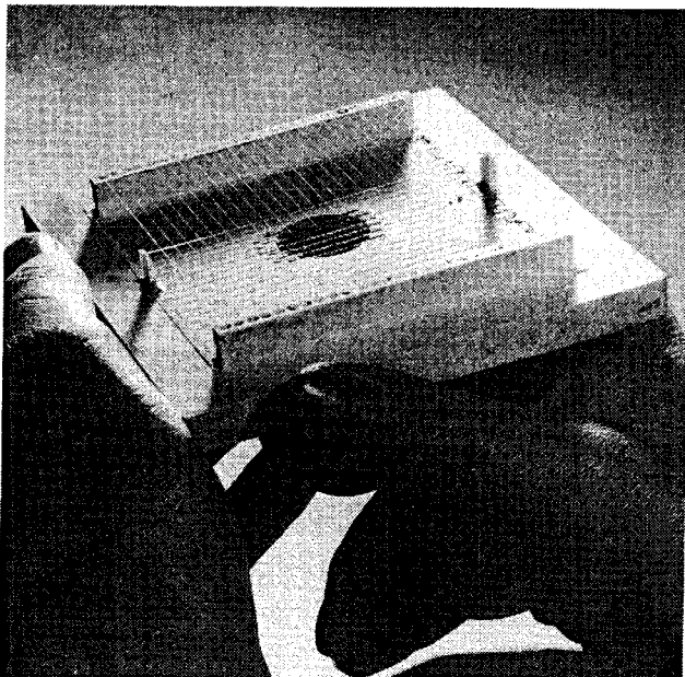
Figure 1. Anode-cathode assembly of the liquid-xenon detector. Anode wires (5 \mu diam.) and cathode strips are spaced 2.8 mm apart. Wires are centrally supported by passing between two quartz fibers.
