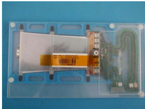
Figure 2.18 A module that passed the electrical readout tests at the University of Geneva packed in a transport box before being shipped to CERN.
