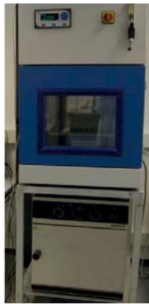
Figure 2.2 The climate chamber used for thermal cycling of the module.
