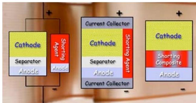
Polymer "shorting agents" can redirect the flow of current when a battery is fully charged. Reversible shorting agents can be used outside the cell (left), as an extra internal component of the cell (middle), or as a composite in the separator between anode and cathode (right).
