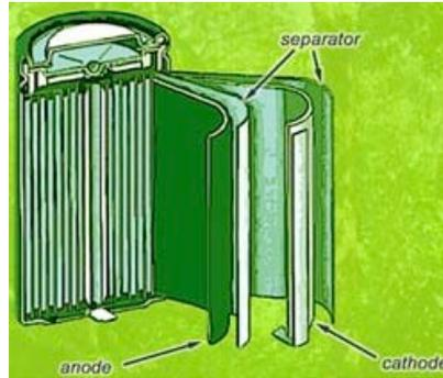
One technology with great promise for future electric vehicles is the light-weight, high-voltage lithium-ion battery widely used in today's electronic devices.
