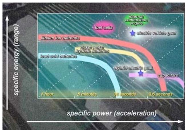
A map developed by Venkat Srinivasan from product fact sheets compares the specific energy (in watt-hours per kilogram) of vehicle power sources, an indicator of their range, with their specific power (in watts per kilogram), an indicator of acceleration. Dotted lines indicate acceleration and cruise times, while blue stars show DOE's energy and power goals for electric vehicles and hybrids. Internal
