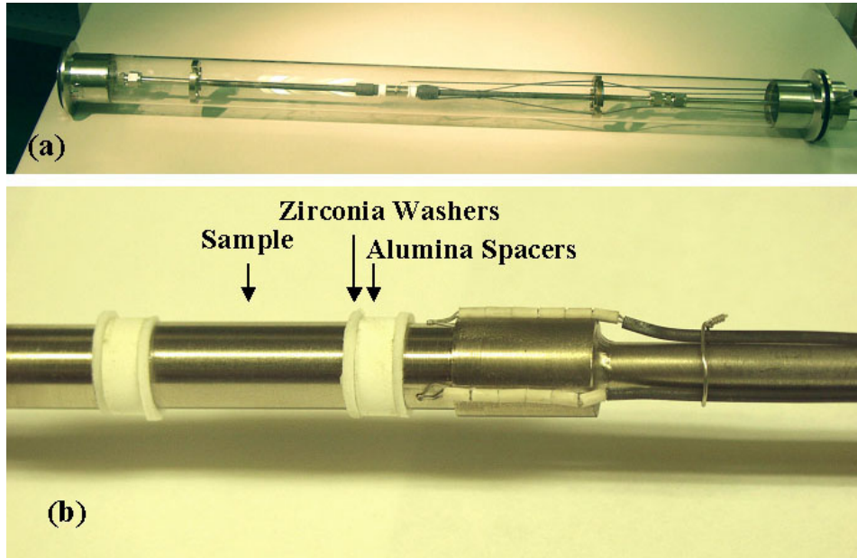
Figure 8. Test train for conducting one-sided steam-oxidation kinetics tests in-cell using \approx 25 -mm-long Zircaloy cladding samples: a) test train within quartz tube; and b) enlarged view of sample region along the test train showing alumina spacers to inhibit Zircaloy-Inconel interaction and zirconia washers to minimize steam leakage to the sample inner surface.
