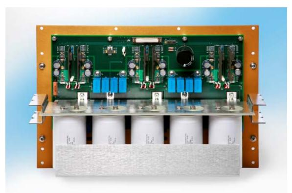
Photograph 3 - Bridge Matrix Assembly, front (One of four used in the 500kW inverter)
