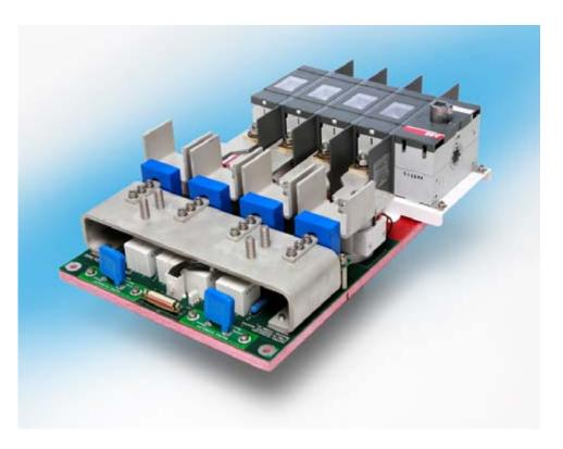
Photograph 8 - PV Interface Assembly
