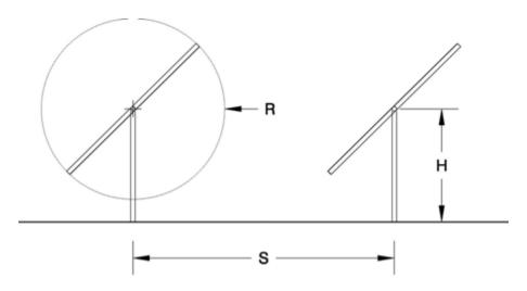
Figure 16 – Programmable Array Form Factor Parameters
