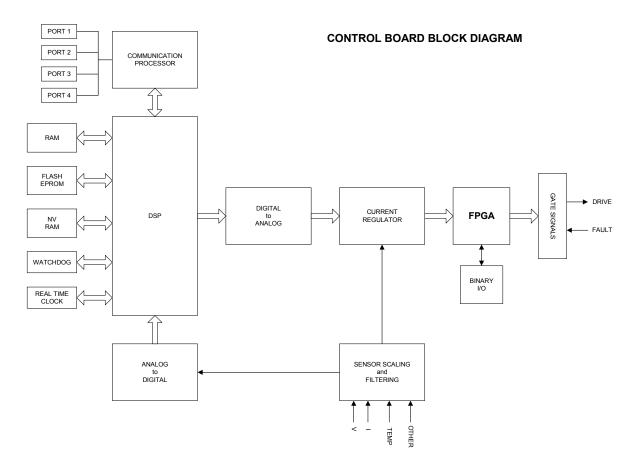
Figure 6 - DSP Control Board Block Diagram
