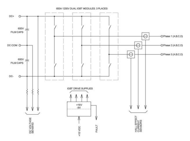
Figure 3 - Bridge Matrix Assembly Schematic Diagram
