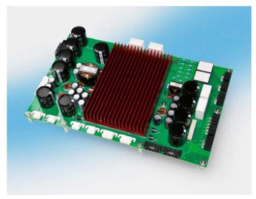
Photograph 5 - Power Supply Board Assembly
