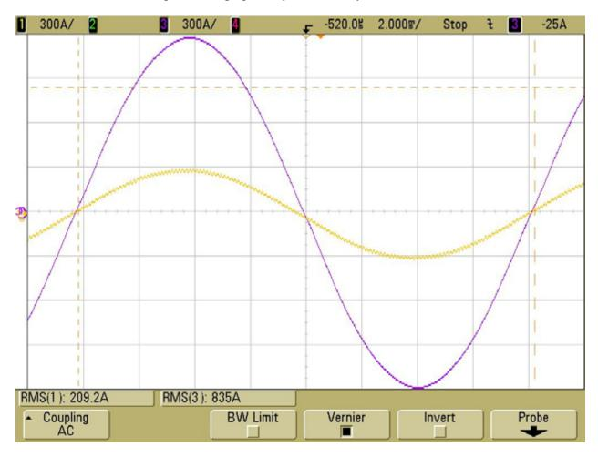
Figure 18 - Full Current Operation at Maximum DC Voltage
