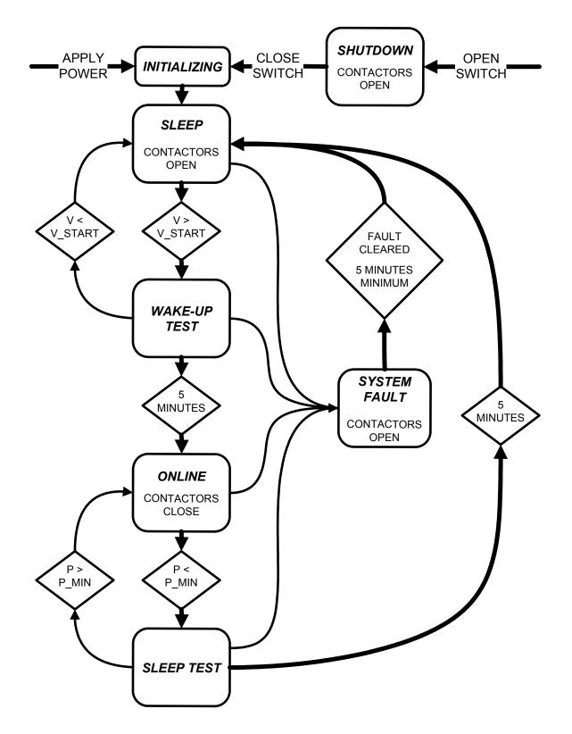
**Figure 13 - State Machine Diagram**
