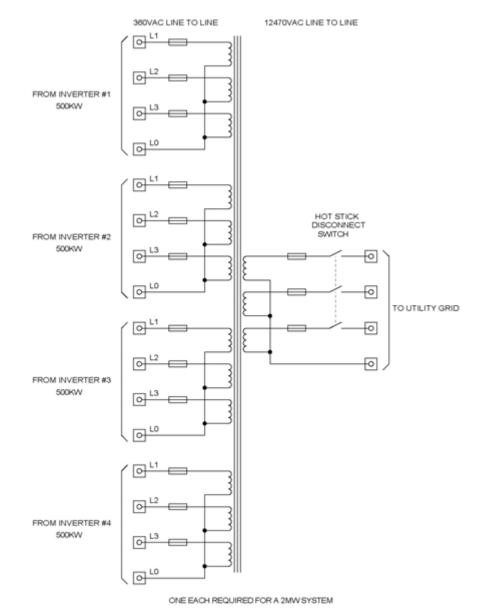
Figure 11 - Solution #3, 2MVA Transformer Subassembly Schematic
