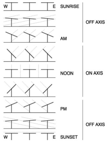
Figure 15 - Tracker Controller Software Anti-Shadowing Algorithm
