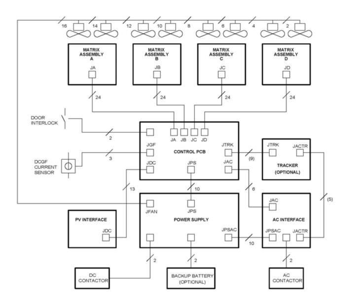
Figure 1 - 500kW Inverter Functional Block Architecture
