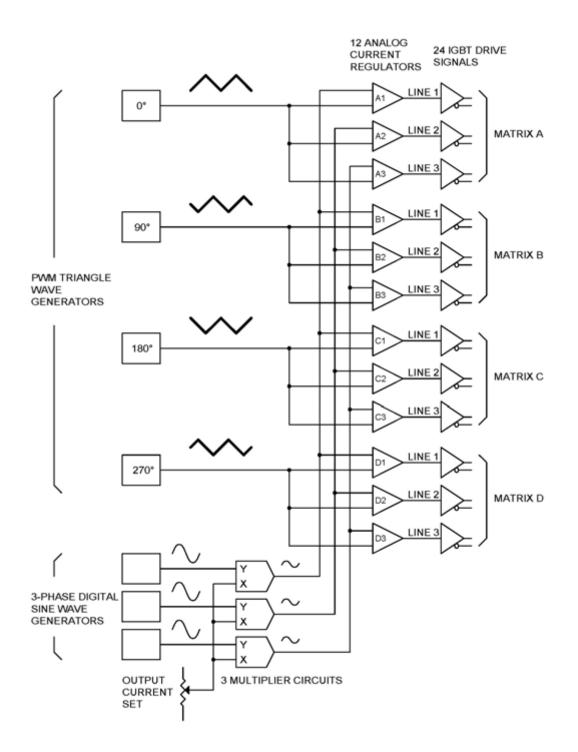
Figure 4 – Analog Control Board Regulation Circuits
