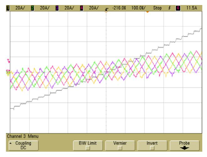
Figure 19 - Interleaved High Frequency PWM Switching
