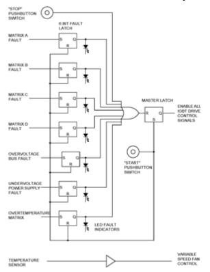
**Figure 5 - Analog Control Board Fault Detection**
