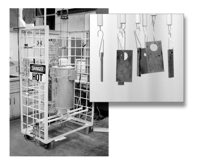
Fig. 3. Cyclic oxidation apparatus for testing in atmospheric pressure steam/air mixtures.
