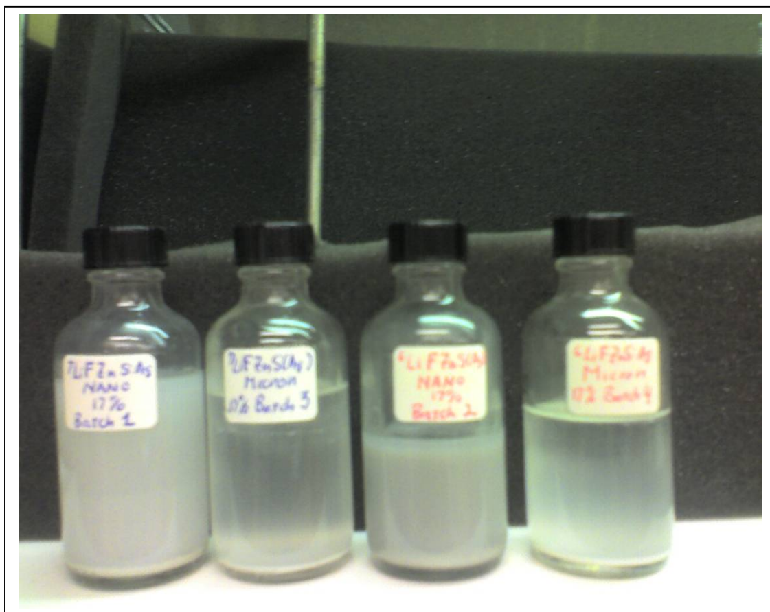
Figure 13. Bottles containing the LiFZnS/Polystyrene/Toluene solution fabricated in batches (left to right) 1, 3, 2, and 4 after 8 days of settling.
