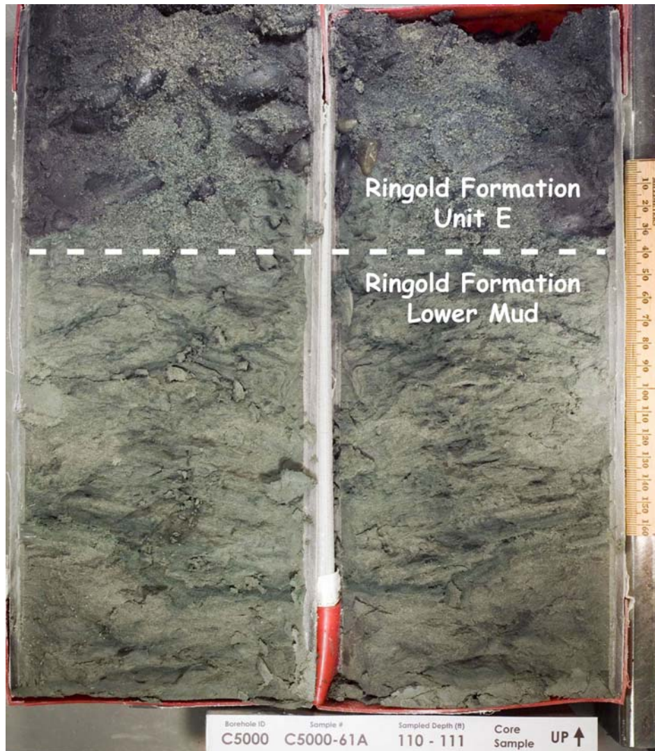
Figure 3.10. Core Photograph Showing the Ringold Formation Unit 5 and Unit 8 Contact Boundary in Well 399-1-23 (C5000)
