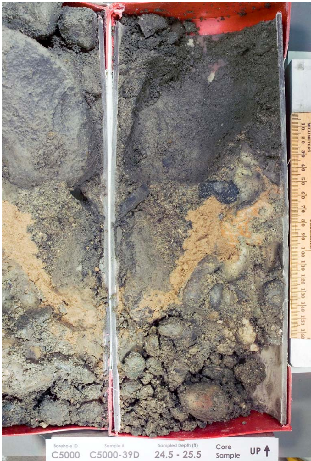
Figure 3.20. Core Photograph Showing Reworked Sediments Within the Hanford Formation Vadose Zone in Well 399-1-23 (C5000)
