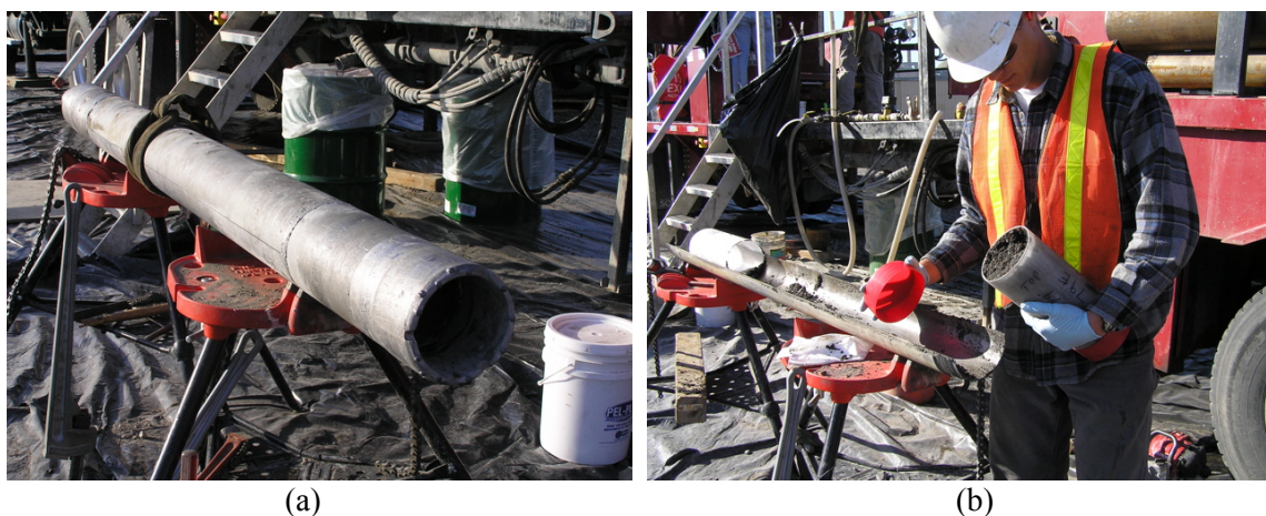
Figure 6.2. a) Six-Foot Splitspoon Core Barrel and Drive Shoe, and b) Opened Splitspoon Core Barrel During Recovery of Lexan Core Liners
