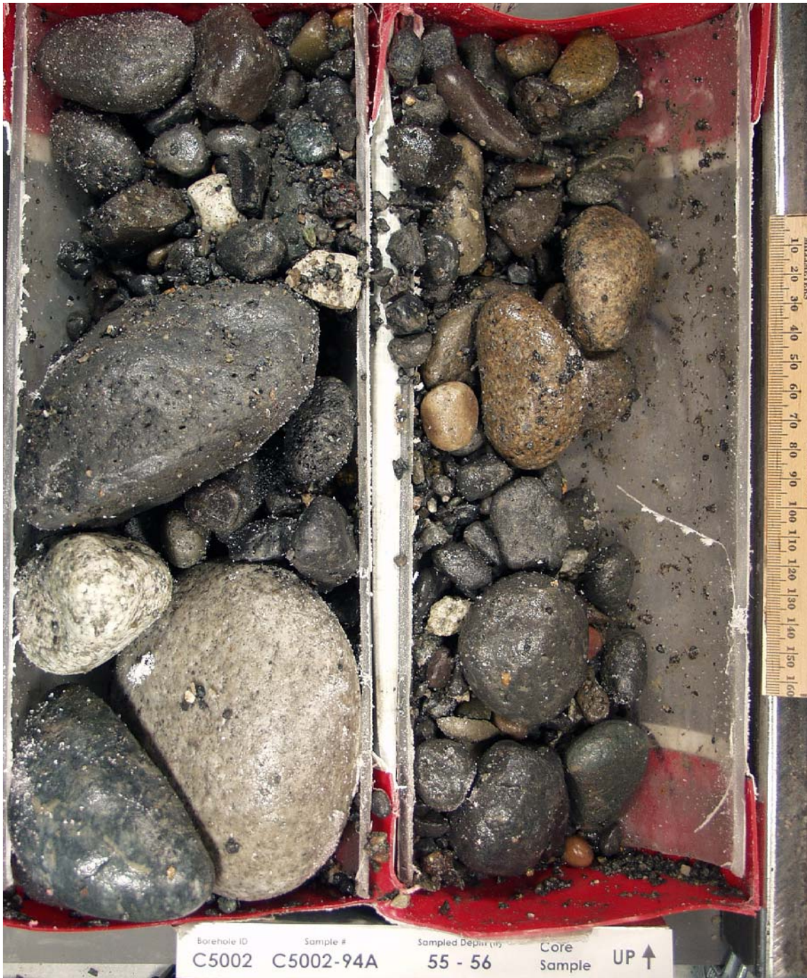
Figure 3.19. Core Photograph Showing Open-Framework Gravel of the Hanford Formation in Well 399-3-20 (C5002)
