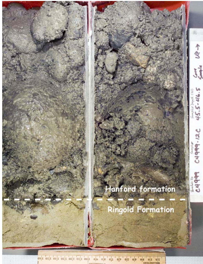
Figure 3.9. Core Photograph Showing the Hanford Formation - Ringold Formation Contact Boundary in Well 399-3-18 (C4999)
