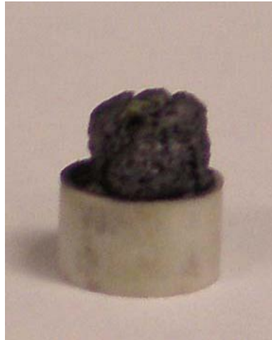
Figure A3. LSM precursor in alumina crucible after DSC-TGA run. The precursor filled \sim 1/5^{\text{th}} of the crucible prior to heating.
