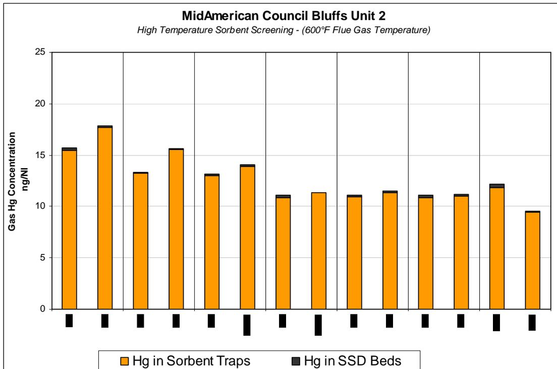
**Figure 1. MidAmerican CBEC Unit 2 High-Temperature Sorbent Screening Results.**
