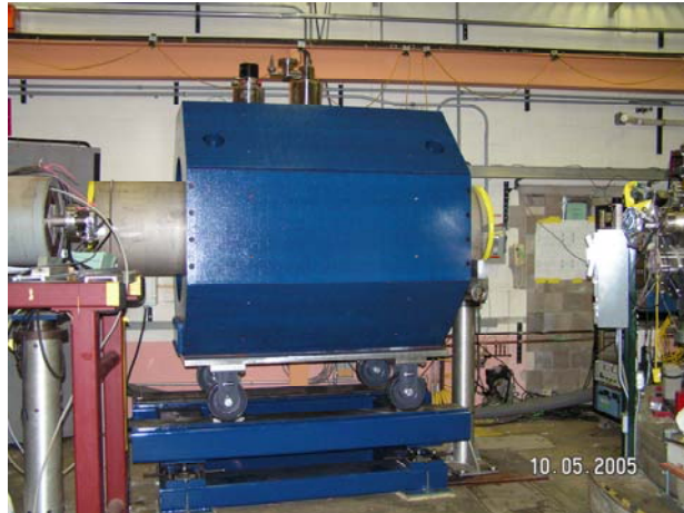
Fig. III-49. The large 65 cm bore 1.5 T superconducting solenoid inside its passive iron shield installed in location on its support structure in experimental area II.
