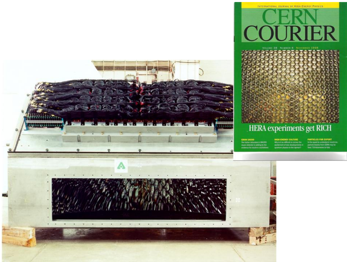
Fig. IV-18. Front view during installation of the upper section of the HERMES RICH detector with the aerogel wall removed. The image of the photon detector matrix is visible in its reflection in the mirror array. The inset shows a cover of the CERN courier which contains a picture of the pmt matrix.
