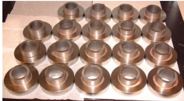
Fig. III-5. Group of three center conductors set up in the electron beam welding chamber for seam welding halves together (left). Mass production of niobium to stainless steel braze transitions (right).
