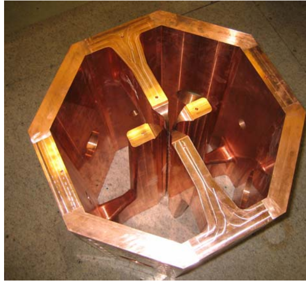
Fig. III-9. Top view of the pre-brazed assembly of the RFQ cavity.
