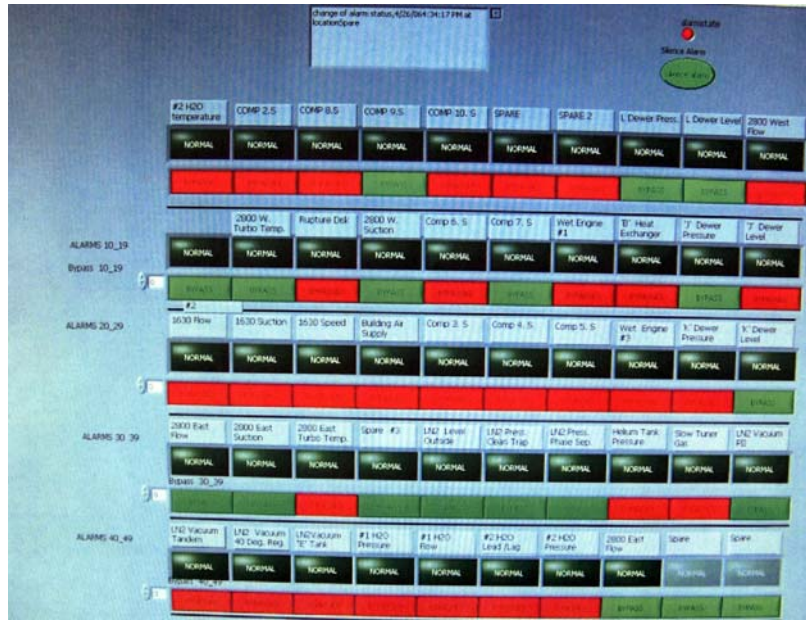
Fig. II-7. The new cryogenic alarm system control screen.
