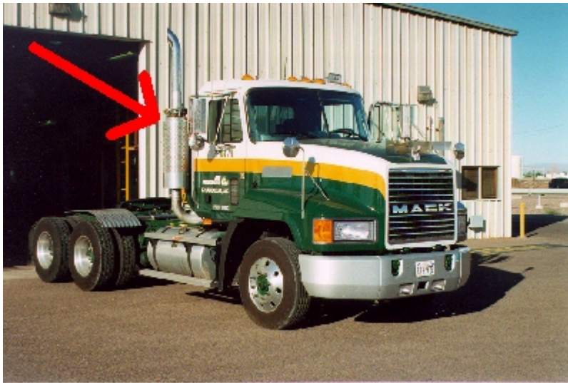
Figure 4-7 1kW TEG equipment using the waste heat from a truck built by Hi-Z
