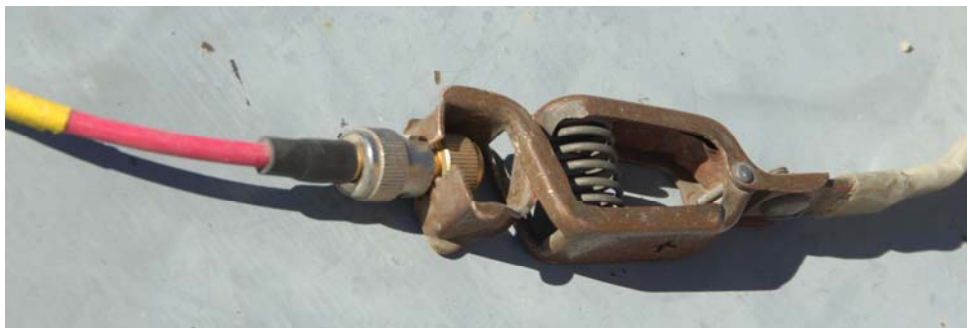
Figure 16. Shunting Plug Ground Connection
