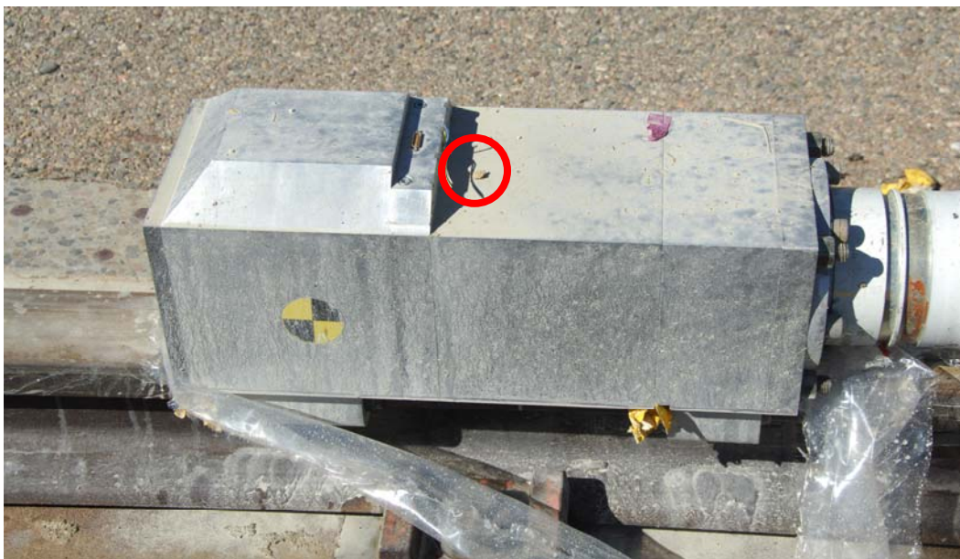
Figure 18. HiCap Recorder Showing Loose Signal Wires
