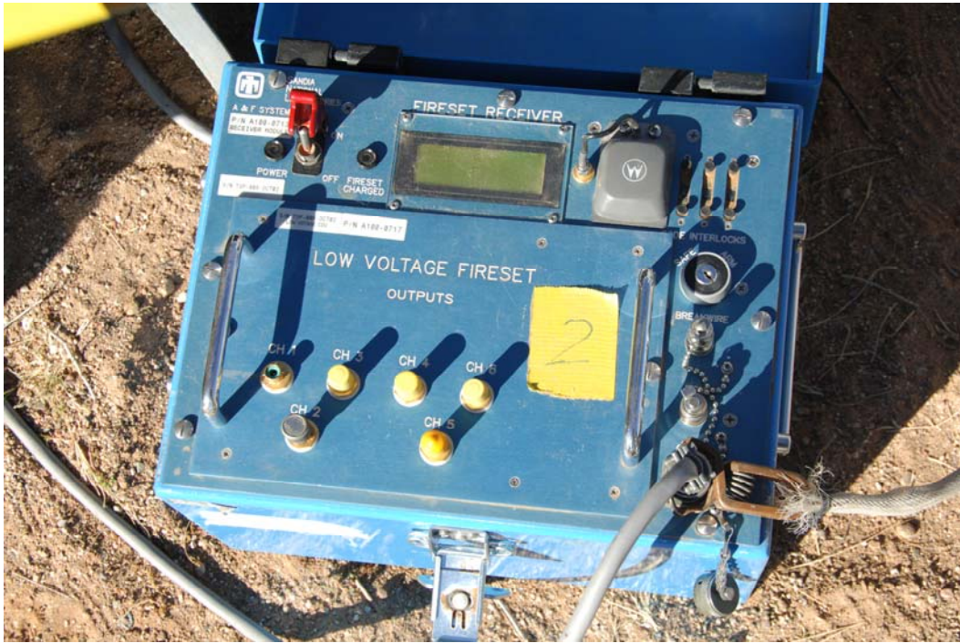
Figure F-1. Fire Set Planned for Use to Initiate Rocket Motor Initiators
