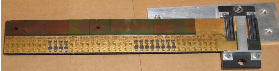
Figure 6 Early prototype ladder equipped with MAPS. A Kapton cable with 4 copper conductor layers was used to route signals from/to sensors to the edge of the ladder. Analog buffers are visible at the edge of the ladder.
