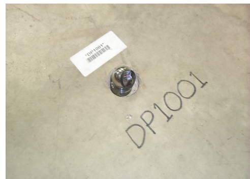
(c) Spherically-Mounted Rectroreflector (SMR) mounted on a brass plug
