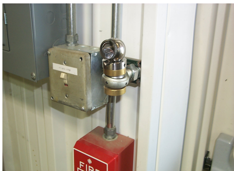
(b) A SMR mounted on a tie rod and a tie adapter
