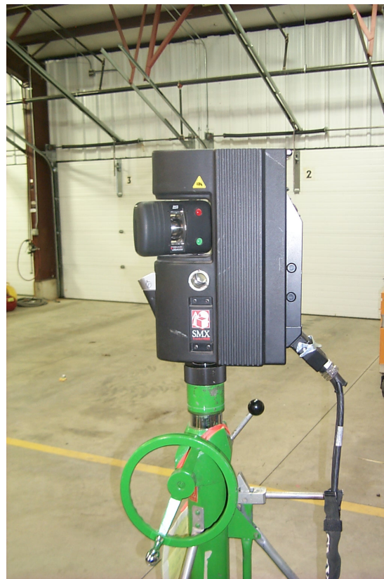
Figure 5.4: An actual laser tracker SMX 4500 in use for survey work at Fermilab
