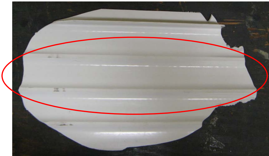
Figure 11: PVC piece from the extrusion
