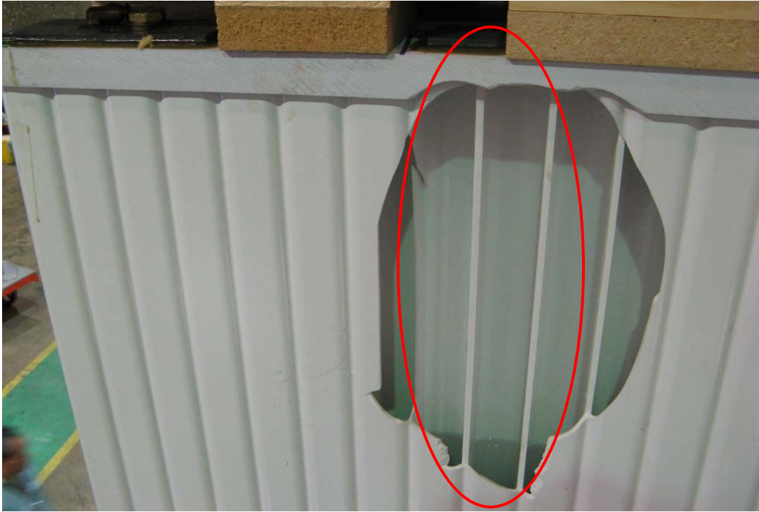
Figure 12: Fracture on the extrusion
