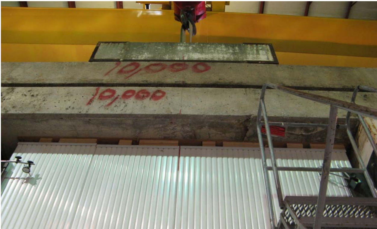
Figure 7: Put the 12 ton weight blocks on top of the IPND prototype
