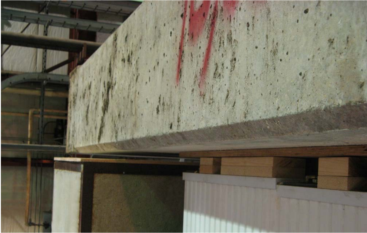
Figure 6: Put the first 5 ton weight block on top of the IPND prototype
