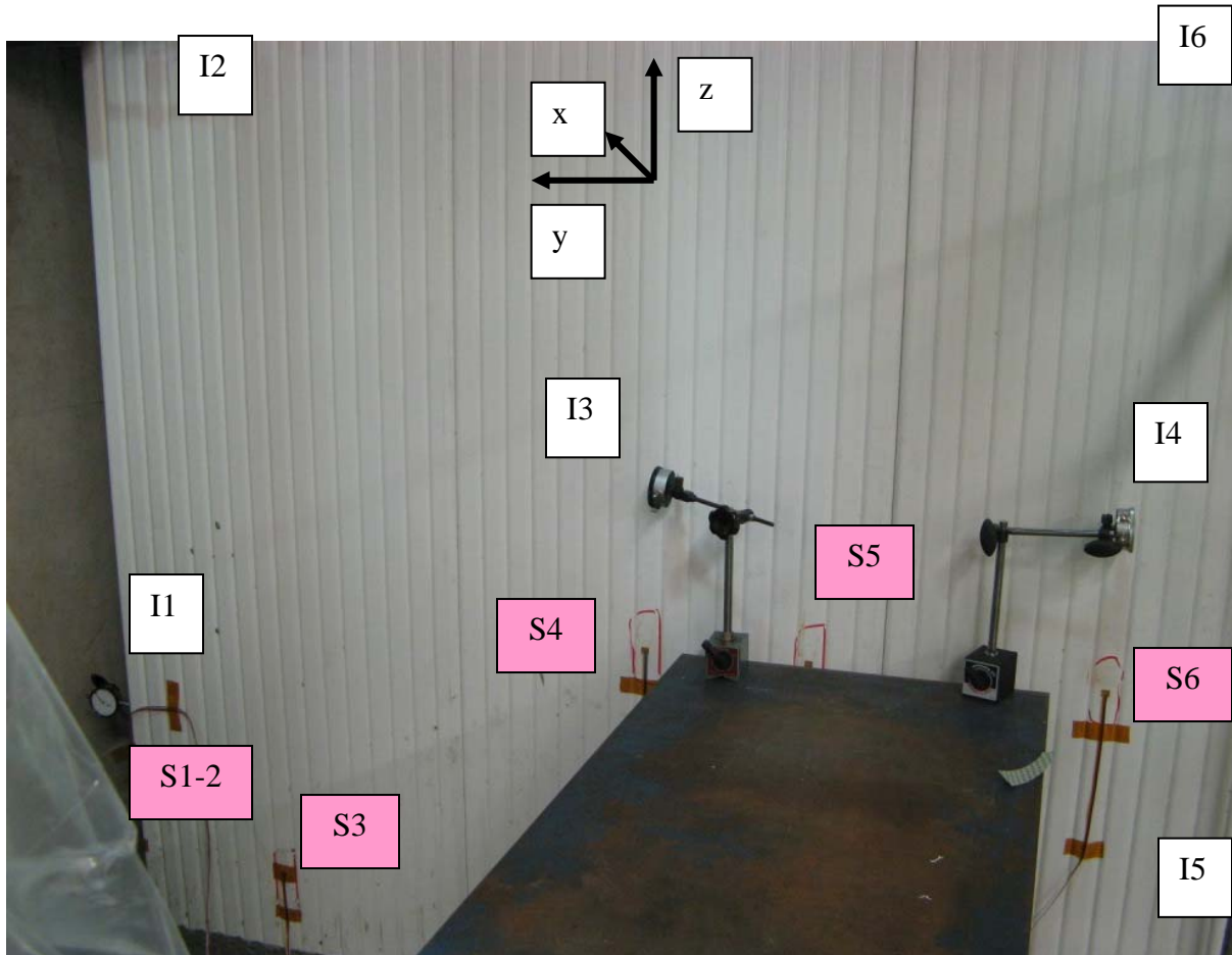
Figure 4: Layout of strain gages and dial indicators on the IPND Prototype
