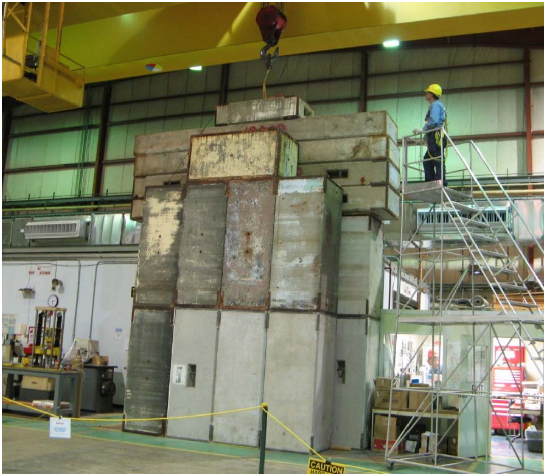
Figure 8: Put the 22 ton weight blocks on top of the IPND prototype
