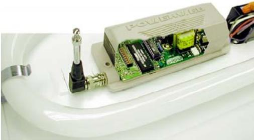
**Figure 13.** Application-specific controller produced by Power Web Technologies. The addressable controller can control one relay and two 0-10 VDC analog dimming ballast loops. A wireless network communicates with the controller through the RF antenna shown at the left.
