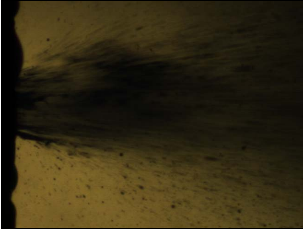
Figure 13. A sample image of a water spray taken at 16 \mu s exposure. Nozzle conditions: 5 kg/hr water, 0.95 kg/hr air at 18 psig.
