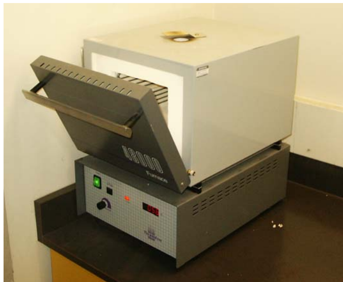
Figure 11. Furnace used for smelt properties testing.
