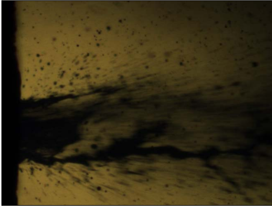
Figure 15. A sample image of a water spray taken at 16 \mu s exposure with the fluid and air connections reversed. Nozzle conditions: 5 kg/hr water, 0.44 kg/hr air at 40 psig.
