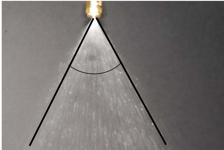
Figure 49. Spray from a full cone nozzle at 2 liters/min, Spray angle: 50^\circ .
