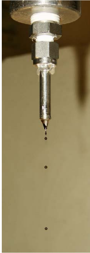
Figure 26. Tip of the prototype droplet injector and resulting droplet stream.
