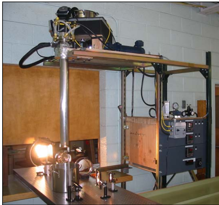
Figure 5. Experimental setup for backlit images of the liquid spray.
