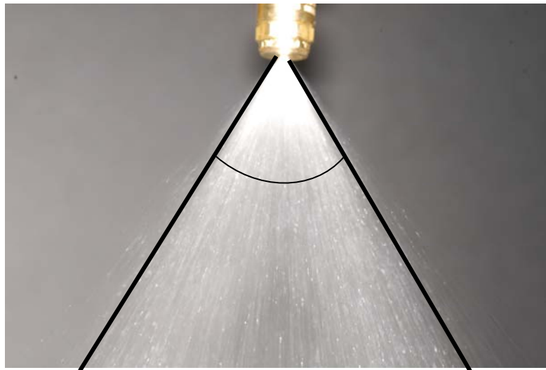
Figure 50. Spray from a full cone nozzle at 3 liters/min, spray angle 62^\circ .
