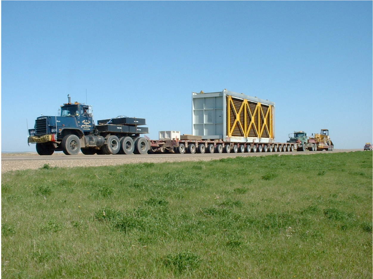
Figure 25. Transporting Part of Waste-Heat-to-Oil heater Assembly during Spring Load Limit Restrictions. (Transport device uses 18 double-axes)
