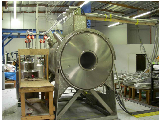
Fig. 3. Finished Spectrometer Solenoid 1 before the Magnet Cool-down
