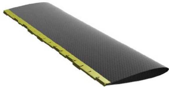
Fig. 3-19 Concept wing with MiTEs. (Source: Bieniawski et al. 65 )
