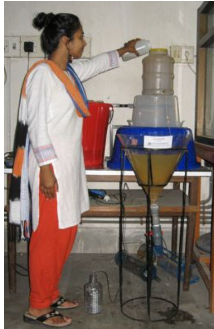
Figure 44: Shefah Qazi Tests the 10 liter per hour Prototype Clarifier
