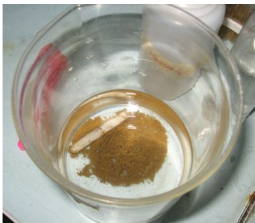
Figure 46: Coagulated ARUBA Particles, Ten Minutes after Addition of the Polyelectrolyte
