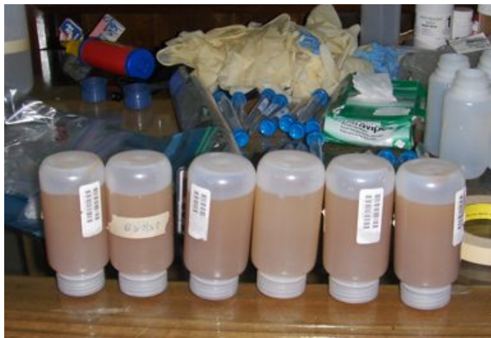
Figure 9: Maintaining Particle Suspension during a Capacity Test in Bangladesh
