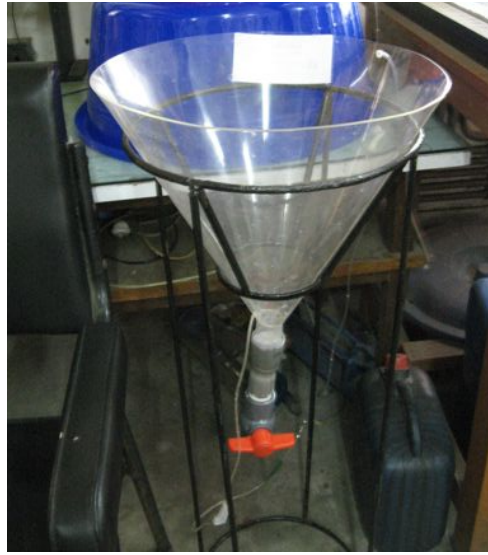
Figure 43: Ten Liter per Hour Prototype Clarifier
