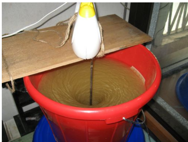
Figure 38: Electric Kitchen Mixer Mixing ARUBA into 20 Liters of Contaminated Water
