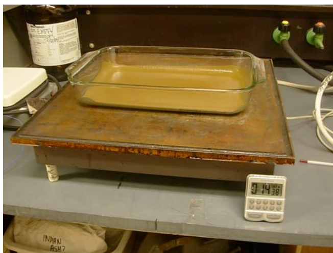
Figure 8: ARUBA Drying in a Pyrex Dish on a Hot Plate
