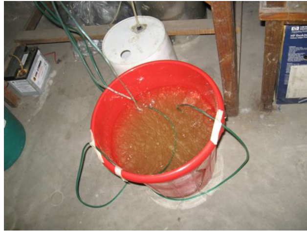
Figure 36: Aeration Pumps Mixing ARUBA into 20 Liters of Contaminated Water
