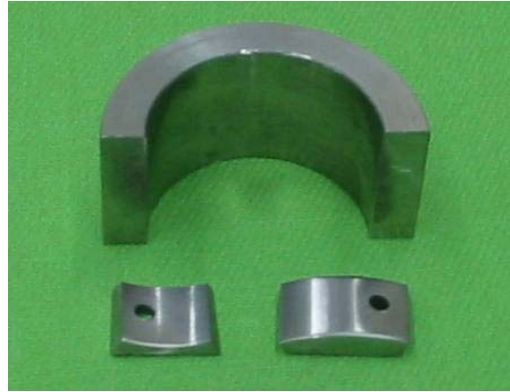
Fig. 1. Section of Save12 10.5Cr pipe (2-in O.D.) and curvature samples cut from pipe. All but one side of the curvature samples are flat. Samples: concave (left) and convex (right).
