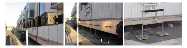
Figure 17: Time reversal array system of 8 speakers (left), 8 microphones (center), arranged in two horizontal arrays (right).
